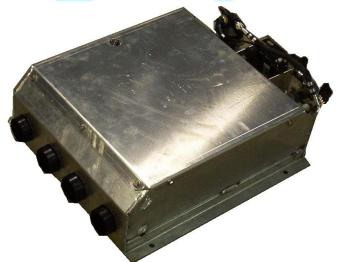
driven AC systems to keep you cool. *If it keeps the Navy cool, it can keep you cool, too.* These 12 or 24 Volt systems produce 24,000 BTU of cooling and 30,000 BTU of heat, all in a box that measures 21.5"L x 20"W x 7"H. Small enough to be installed underneath flooring or behind bulkheads, this unit provides 600 CFM to 4 vents that can be installed around a cabin, as required.
